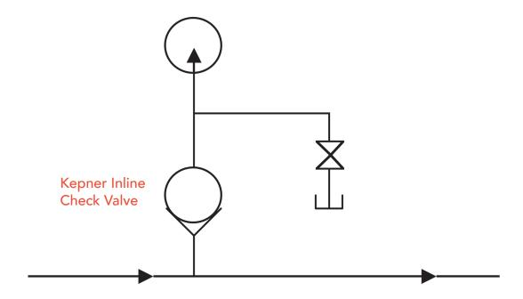
The simple circuit shown above is an integrator for use in cases of repetitive shock or single surges of duration within the response rate of the gauge. On each successive pressure rise an increment of fluid is trapped in the gauge line until the gauge line pressure balances the surge pressure. When the gauge reading stabilizes, the reading will be very close to the peak surge pressure.
